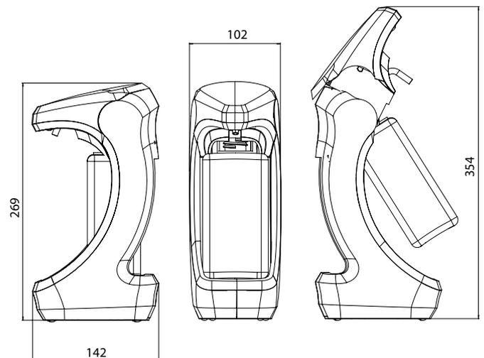
RX 5 T | Abmessungen in mm
